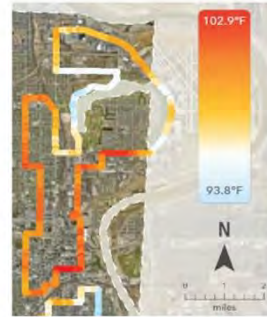
Evening Routes (7 – 8 p.m.) Over 15,000 unique temperature measurements are displayed on this portion of our study area. Temperatures vary from coolest (93.8°F) to warmest (102.9°F).
